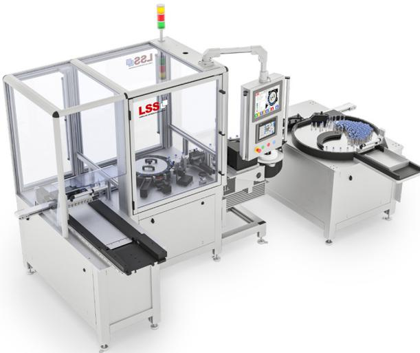
The In-line model extended to include buffer table and tray outfeed system
